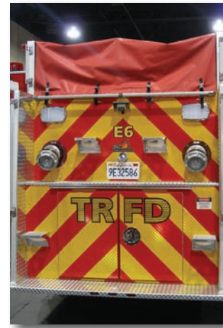
Figure 3.23. Newer fire apparatus are required to have chevron markings on the rear of the vehicle.
