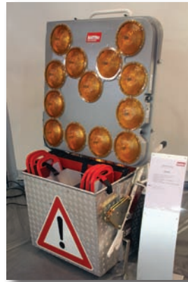
Figure 3.27. Once the cones have been deployed, the traffic arrow may be placed into service.
