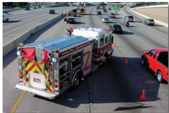
Figure 6.3. First-arriving apparatus should be used to block the incident work zone. Courtesy of Ron Moore, McKinney, TX, Fire Department.
