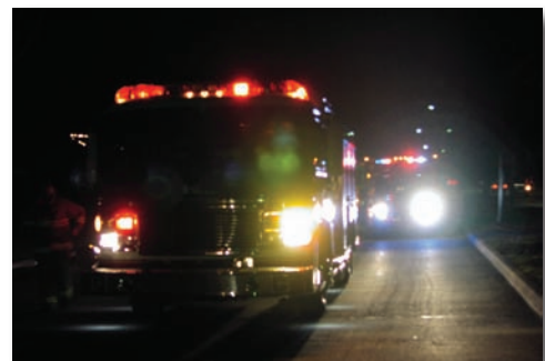
Figure 1.9. Scene light should not be blinding to oncoming motorists. Courtesy of Ron Moore, McKinney, TX, Fire Department.
