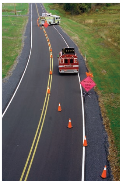
Figure 4.10. A typical TIMA.
