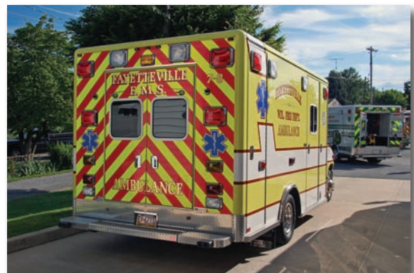
Figure 7.4. Chevrons can be applied to ambulances as well. Courtesy of Jack Sullivan.
