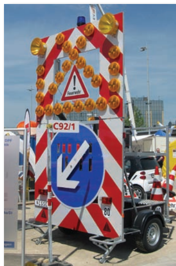
Figure 3.30. This trailer contains a large arrow board.
