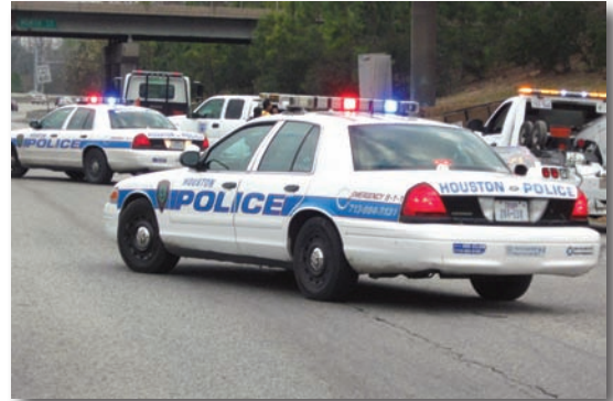
Figure 7.5. Police vehicles may also be used to provide a barrier for the incident work zone.
