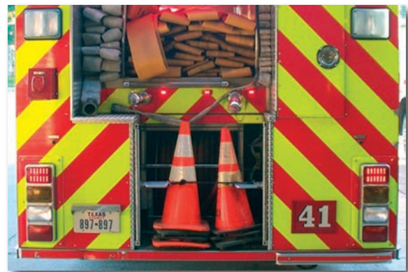
Figure 7.2. All emergency vehicles should carry traffic-control equipment.
