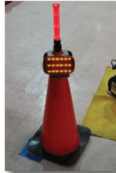
Figure 3.11b. These LED and chemical light stick flares are placed on a traffic cone.
