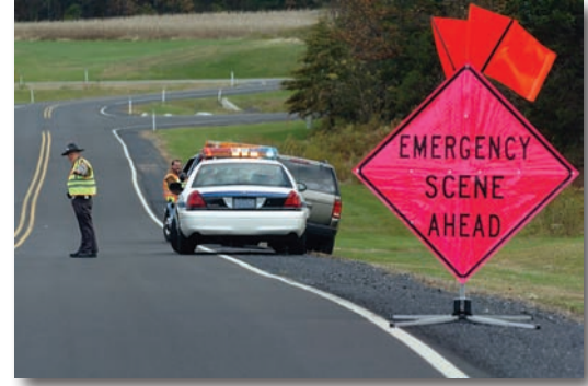
Figure 3.6. “Emergency Scene Ahead” signs should be placed well ahead of an incident scene.
