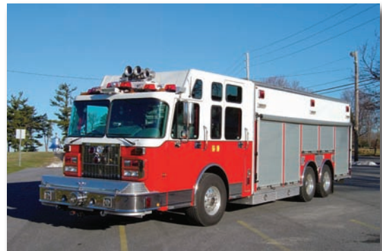
Figure 5.13. Vehicle air horns are one manner in which to notify responders of an evacuation.
