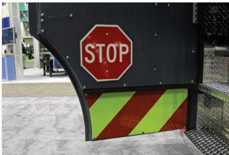
Figure 3.22. This apparatus has reflective markings and a stop sign on the inside of the cab doors.
