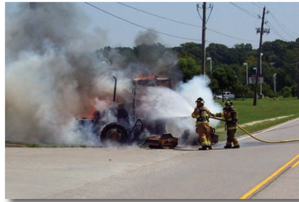
Figure 5.1. All roadway incidents should be operated under the ICS. Traffic safety vests are not required for firefighters wearing a self-contained breathing apparatus (SCBA). Courtesy of Mike Mallory, Tulsa, OK, Fire Department.
