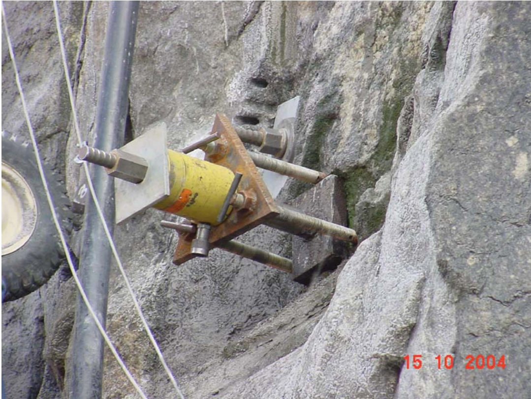
Figure 5. Lift-off Test for Prestressed Rock Bolts
