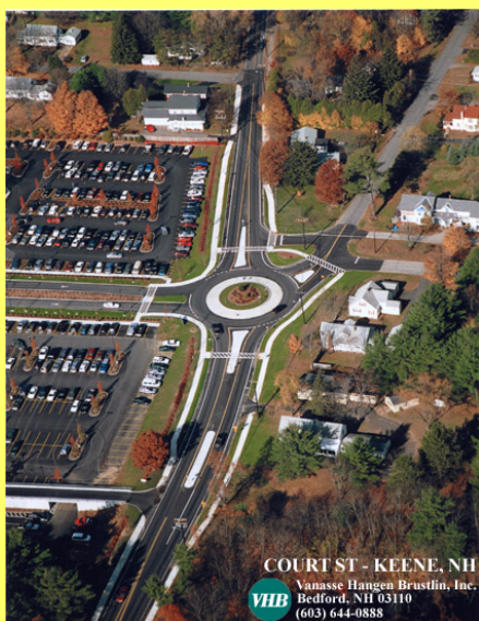
Property Impacts – Because of the smaller size roundabouts usually require less impact to private property than a traffic circle.
