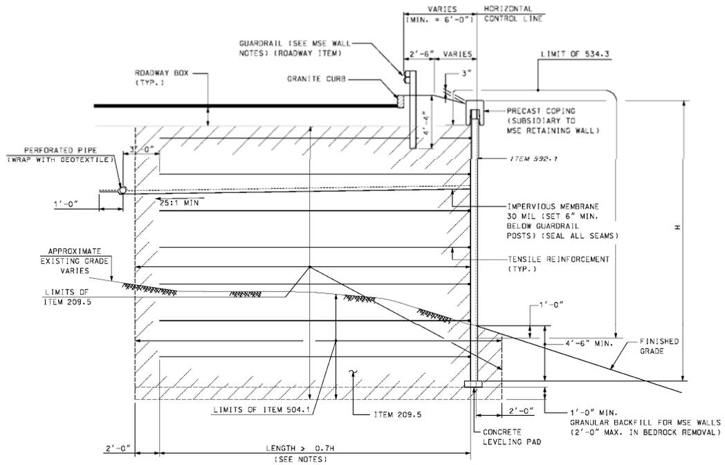
Typical for MSE Wing Wall in Cut with Full Width Layer of Granular Backfill Below Wall
