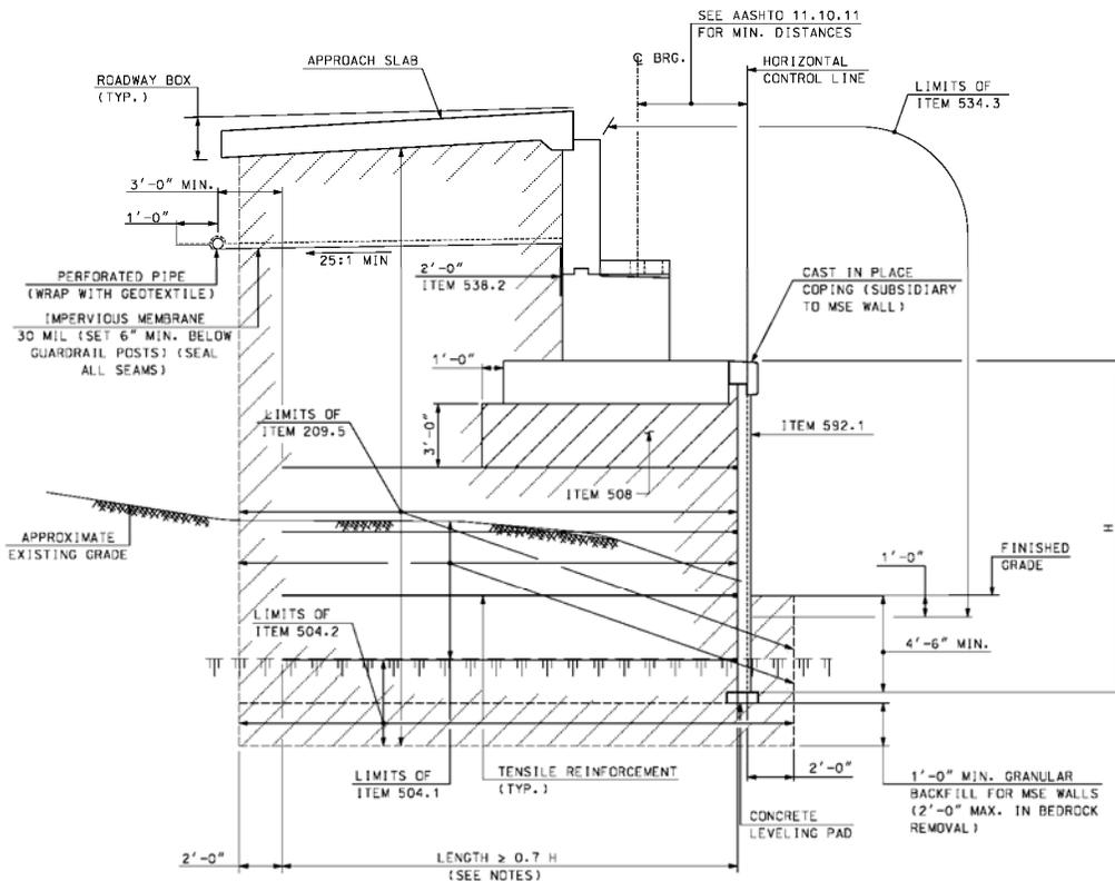
Typical Abutment Section on MSE Wall
