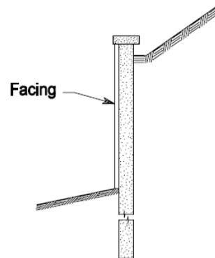
**Slurry or Cylinder Pile
