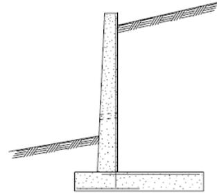
**Reinforced Concrete Cantilever
