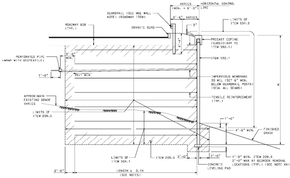
Typical for MSE Wing Wall in Cut with Granular Backfill Below Leveling Pad Only
