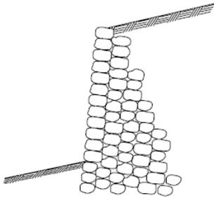
**Mortar Rubble Masonry
