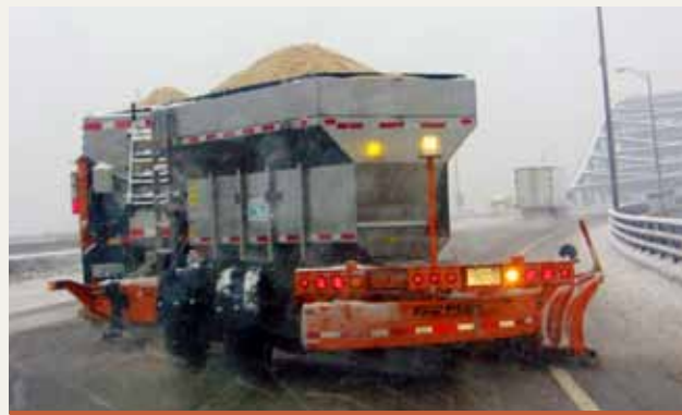
A NHDOT plow truck pulling a tow plow approaches the I-95 “high level” bridge near the Maine state line during plowing operations this past winter.
