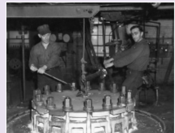
The name of the worker on the right is Roger Dignard. In his comment about this photo, Carl E. Belanger wrote: “This job was referred to as ‘working on the wrenches’.” As he recalls, “The guys on the wrenches would unbolt the cover, swing it open then drop a fill chute down so that [wood] chips could be poured into the digester.”
